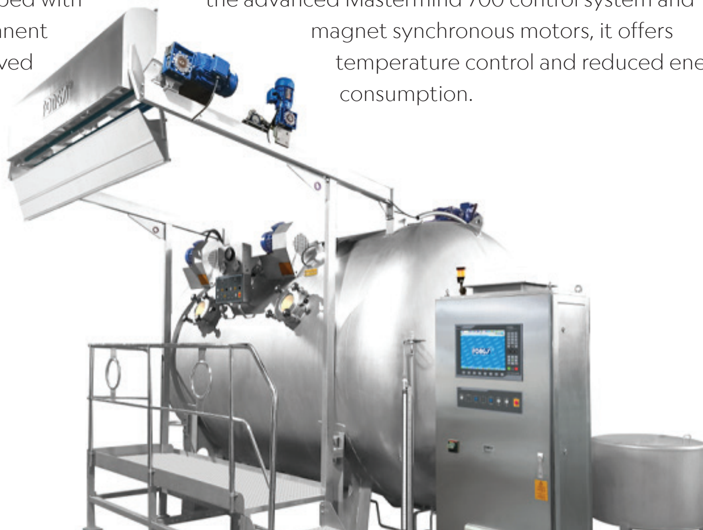
Photo: SOFTWIN High temperature overflow dyeing machine.
